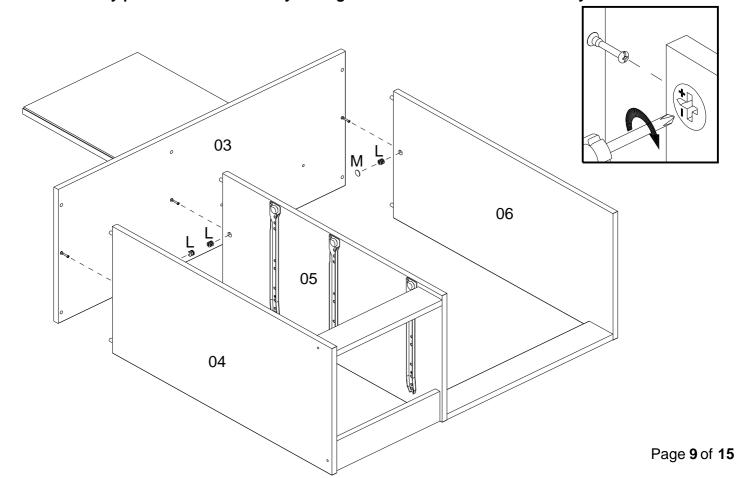
**Step 16:** Attach the small plastic foot (E7) with the hardware N in the left side (04), and division (05), and right side (06) using a small mallet (not provided).
