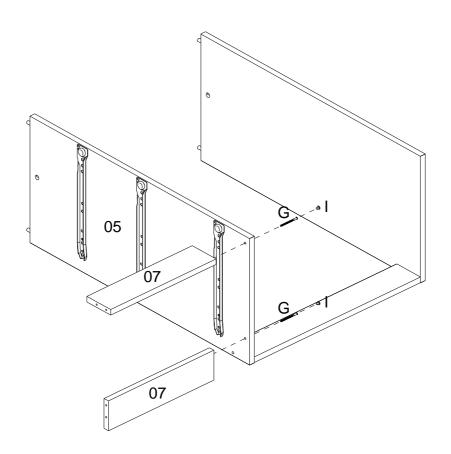
**Step 12**: Attach the left side (04) to the footer module drawers (07) using the hardware G, H and I. **DO NOT use any power tools as this may damage the frame and will invalidate any claim.**
