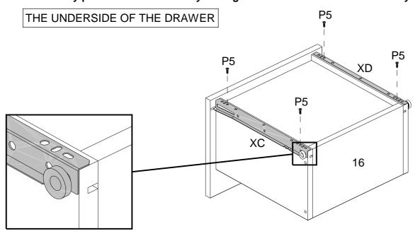
**Step 27:** Join the drawers to the assembled section.
