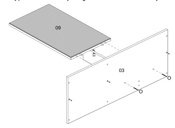
**Step 15**:Attach the assembled section using hardware part L in the left side (04), and division (05),and hardware part L and M in the right side (06) using the a screwdriver (not provided).
