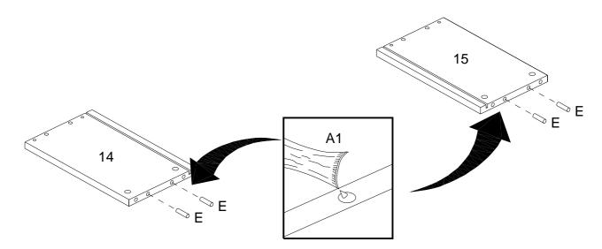
**Step 5:** Attach hardware part E the mirror panel (09) and to the mirror platter (10) using small mallet (not provided). Attach hardware part A3 the mirror platter (10). **DO NOT use any power tools as this may damage the frame and will invalidate any claim.**
