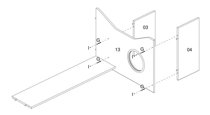
**Step 13:** Join the lower right side (14) to the shelf (03) and bottom base (04) using hardware part G, H and I. **DO NOT use any power tools as this may damage the frame and will invalidate any claim.**
