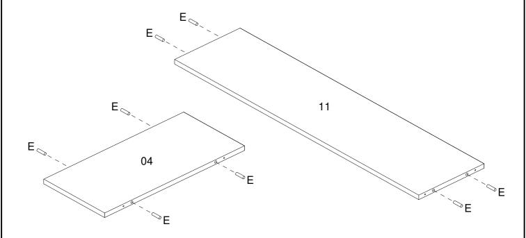
Step 3: Insert hardware part E using small mallet (not provided).
