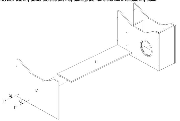
**Step 15:** Join the top (16) to the lower left side (12), lower division (13) and lower right side (14) using hardware part L and a screwdriver (not provided). Insert the hardware part M he lower left side (12), lower division (13) and lower right side (14).
