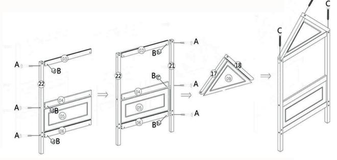
Step 5: Attach he 2 x Side rails (10) and the 2 x Cross bars (11) to the 1 x Front right leg (1), 1 x Back right leg (2), 1 x Front left leg (22) and 1 x Back left leg (21) using the hardware parts (A) and (B).Secondly attach the 2 x Support bar (13) and 1 x Roof Cross bar (12) to the 1 x Front right roof panel (7), 1 x Front left roof panel (17), 1 x Back right roof panel (8) and 1 x Back left roof panel (18).
