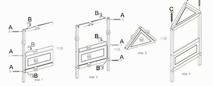
Step 4: Attach the 1 x Front left leg (22) and 1 x Back left leg (21) to the 1 x Top Head rail (3), 1 x Middle head rail (4), 1 x Bottom Panel (5) and 1 x Bottom head rail (6) using hardware parts (A) and (B). Then attach the 1 x Front left roof panel (17), 1 x Back left roof panel (18) and 1 x Top Panel (9) to the 1 x Front left leg (22) and Back left leg (21) using hardware part (C).
