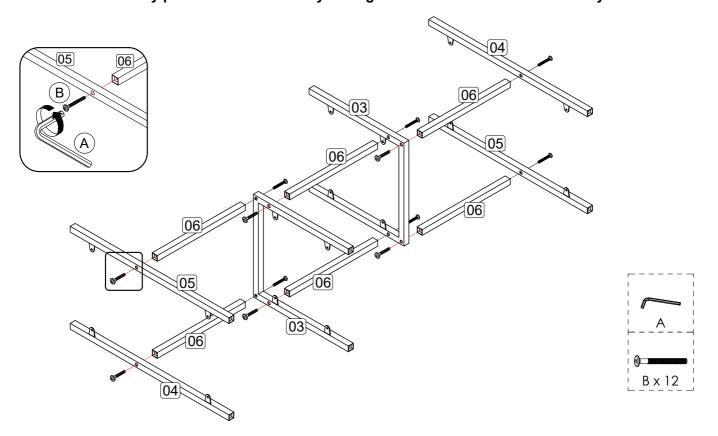
**Step 2:** Attach Metal Side-L (7) and Metal Side-R (8) to Metal Middle (3), Top/Bottom Metal Middle (4) and (5) using hardware A and B.
